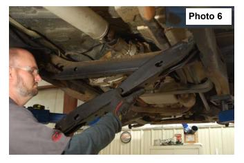
6. Remove the sway-bar using a 13mm socket a pair vise grips on the lower control arm. A 10mm socket and 15mm wrench on the frame. See Photo 7 & 8.
