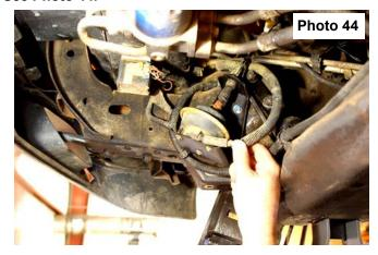
44. Install control arm drop support bar above the stabilizer at this time. Make sure all wires, hoses and cable are above this bar. **See Photo 45.**
