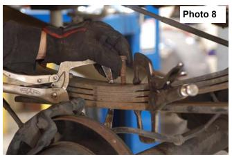
10. Install new spring perch block onto axle. Lower axle onto block. Install the U-bolt top plate on to leaf spring with the short side to the back and install the U-bolts. Install the new lower U-bolt plate using the supplied 9/16" nuts and washers. Tighten using a 22mm socket. **See Photo 9 & 10.**
