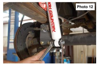
8. Install new brake line ext. onto rear diff using stock hardware and attach the stock brake line bracket to new bracket using the supplied 5/16" x 1 bolt, washers, nut. Tighten using a 13mm socket and wrench. Install emergency brake cable ext. bracket using stock hardware to frame and using the supplied 5/16" x 1 bolt, washer, and nut to attach cable to bracket ext. Use a 13mm socket and wrench to tighten. **See Photo 13 & 14.**
